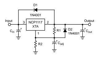
**Figure 22. Protection Diode Placement**
