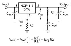
Figure 21. Adjustable Output Regulator
